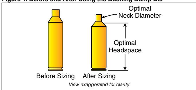
Over 90 interchangeable bushings are available in 0.001" increments. These precision bushings provide great flexibility in adjusting for case neck wall thickness when customizing the neck sizing. See Section 5.0, "Other Applications," for additional sizing options.
